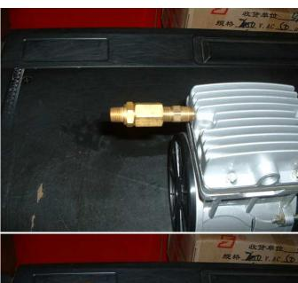
Step 2 – Assemble Female End of Air Saver Valve to Male End of Nipple
