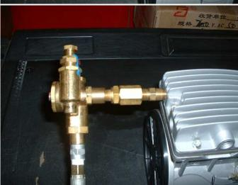
Step 3 – Assemble Female End of DAD-3003 Valve to Male End of Air Saver Valve then Assemble Air Hose to Outlet Port of DAD-3003
