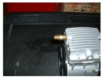
Step 1 -- Assemble ¼ x ¼ Male Nipple to Outlet Port of Compressor
